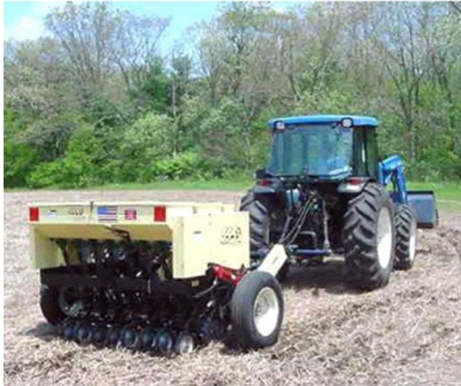
Figure 15. Truax seeder is a no-till drill for warm-season grass seeding. Photo credit: Paul Rothbart.
