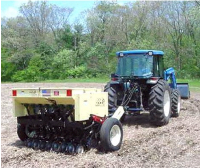
Figure 15. Truax seeder is a no-till drill for warm-season grass seeding. Photo credit: Paul Rothbart.
